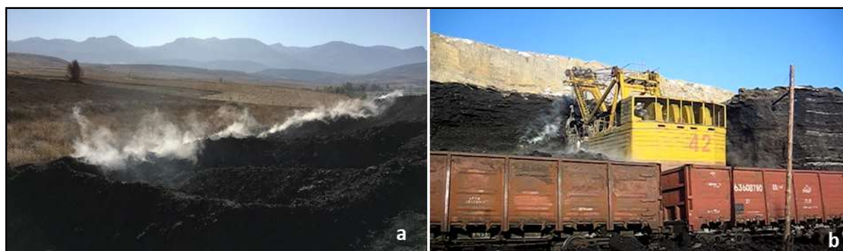
Figure 4. Spontaneous combustion a) in a lignite stockpile in Turkey; b) and in a coal seam in Kazakhstan Presence of chlorine in the form of organic compounds and inorganic forms such as halide minerals and other chlorine containing minerals such as hydrophilite and chloromagnesite can cause severe corrosion in boilers.
